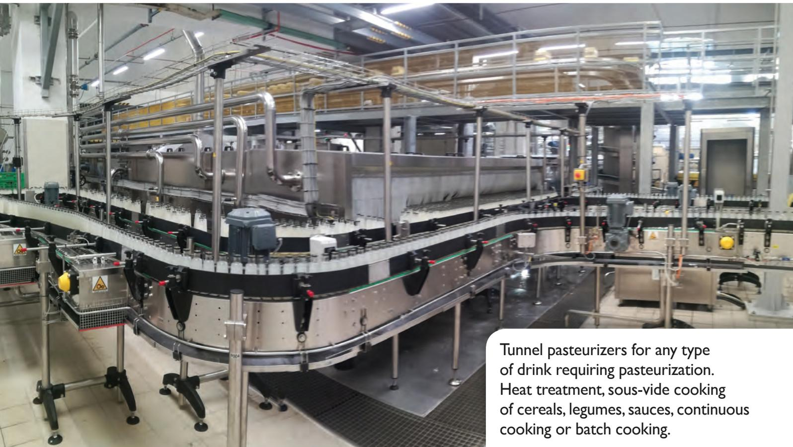
Tunnel pasteurizers for any type of drink requiring pasteurization. Heat treatment, sous-vide cooking of cereals, legumes, sauces, continuous cooking or batch cooking.
