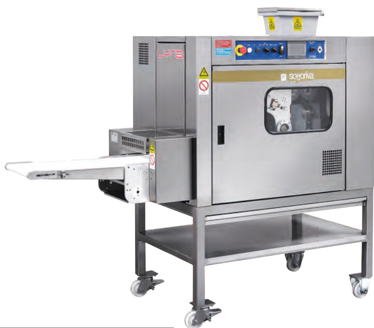
Lyra, divider rounder suitable for medium-small production
