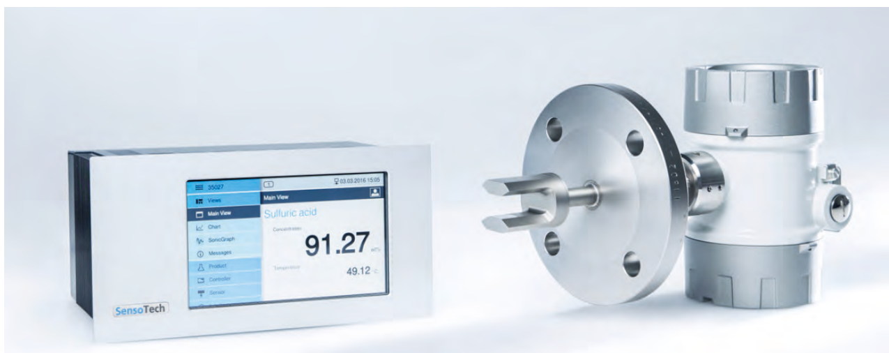
SensoTech's measuring system based on the sonic velocity consists of a forked sensor with electronic housing and a controller as evaluation unit
