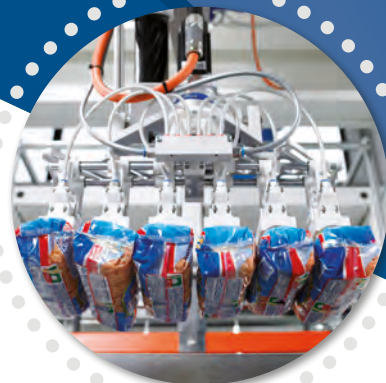
TWIN ROBOT robot for high-speed wrapping of flow pack packages in shrinkable film
