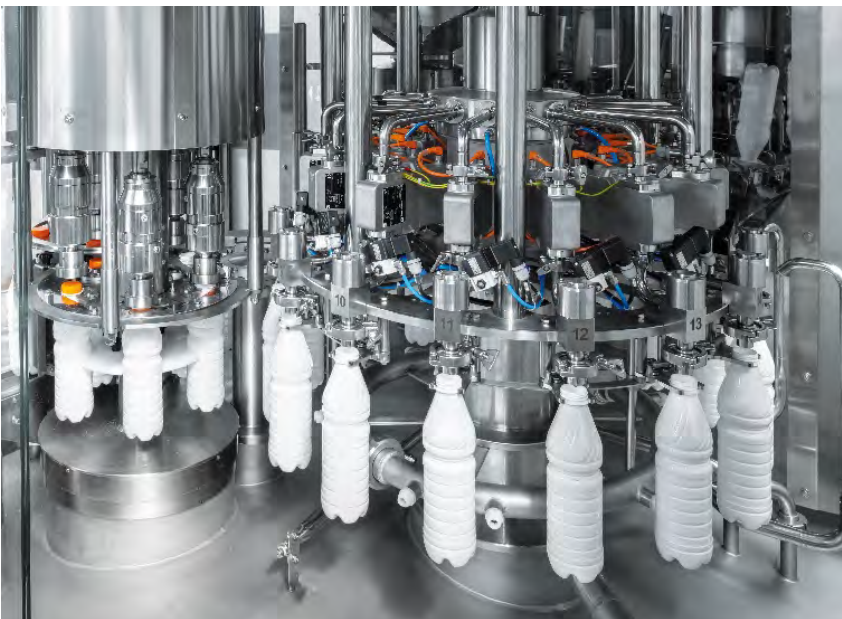
Ultraclean filling carousel with electronic flow meter - contactless filling
