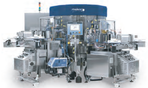
Example of configuration with Roll-Feed stations
