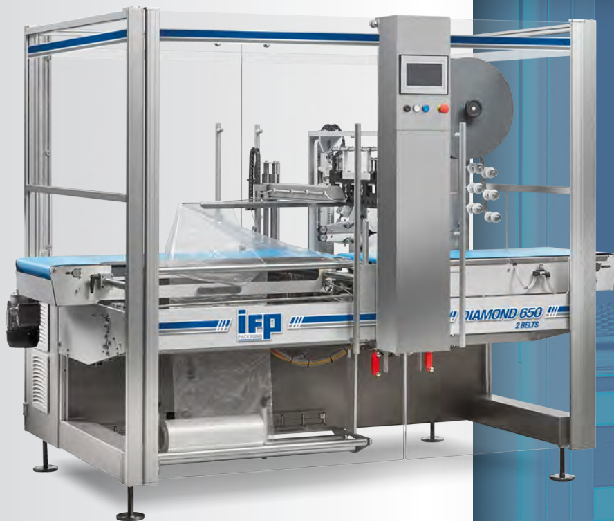
DIAMOND 650 2 NASTRI continuous servo side sealer
