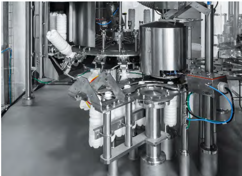
Hydrogen peroxide injection star - for empty bottles sterilization
