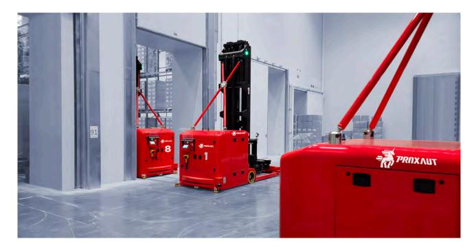
with indoor and outdoor AGV Shuttles. These vehicles are the ideal solution to replace traditional fixed transport systems, gaining in flexibility and configuration of the entire production cycle. Equipped with an adaptable and customizable loading platform and different types of covers, they connect seamlessly to production lines, robotic islands or packaging lines, allowing different types of products to be handled.
