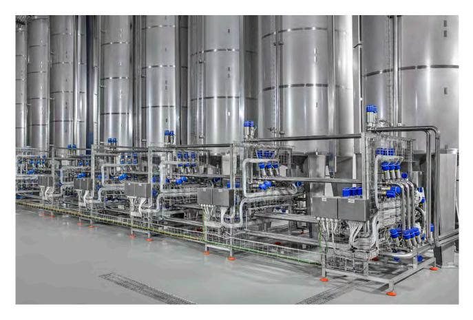
ard modules which are customised for each specific project according to specific needs. Furthermore, the equipment always features a noncompromising technology for what concerns cleanability and hygienic aspects: CIP fluid paths are covering any part of the plant – including process water distribution lines – and the entire piping is tooled to avoid dead legs and minimize the number of weldings. In-house preassembled
