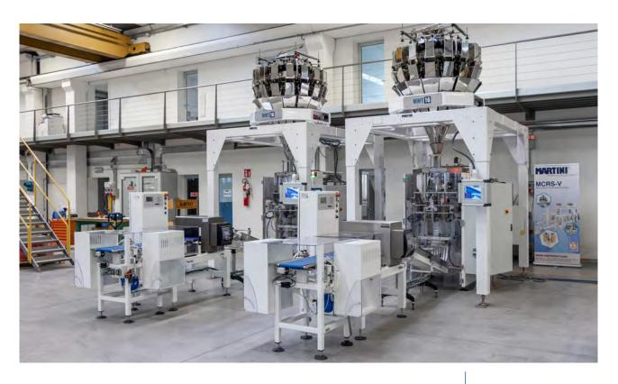
Continous movement vertical packaging machine Model MBM600, reaching 120 bpm, complete with 16-heads multi-head weigher.
