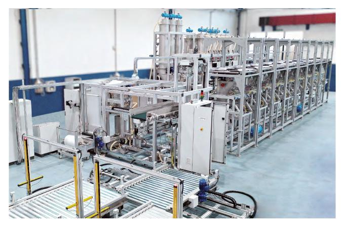
weighing assisted by a PC. In this way, according to the recipe, the system drops the right box and transfer it to the weighing position, where the operator, guided by the PC can dose the product.
