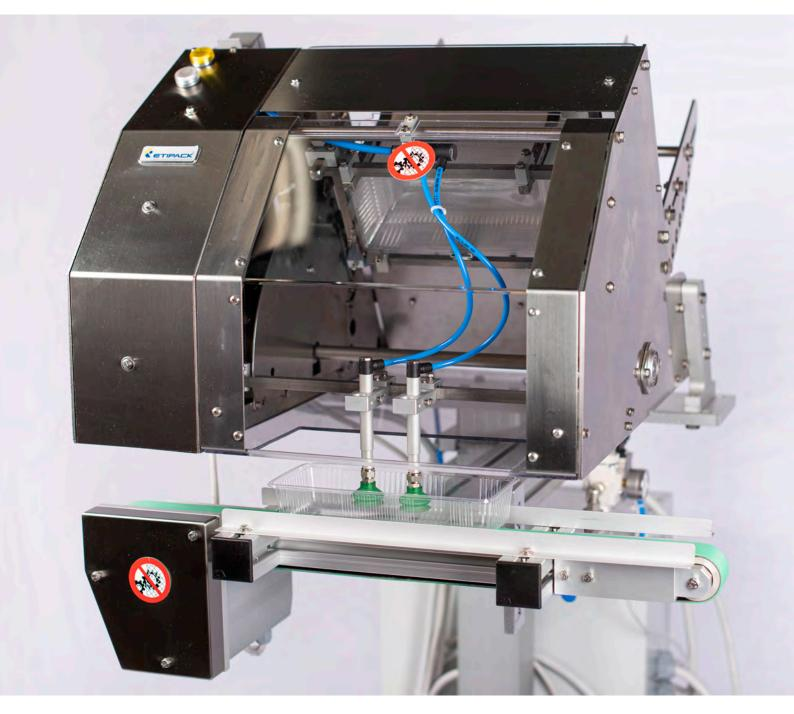
and envelopes up to 3 mm thick, or 8 mm thick with special configuration. It offers numerous configurations for horizontal or vertical processing, as well as the ability to handle formats of various sizes. It also features advanced management of data exchange with the machine and the line.
