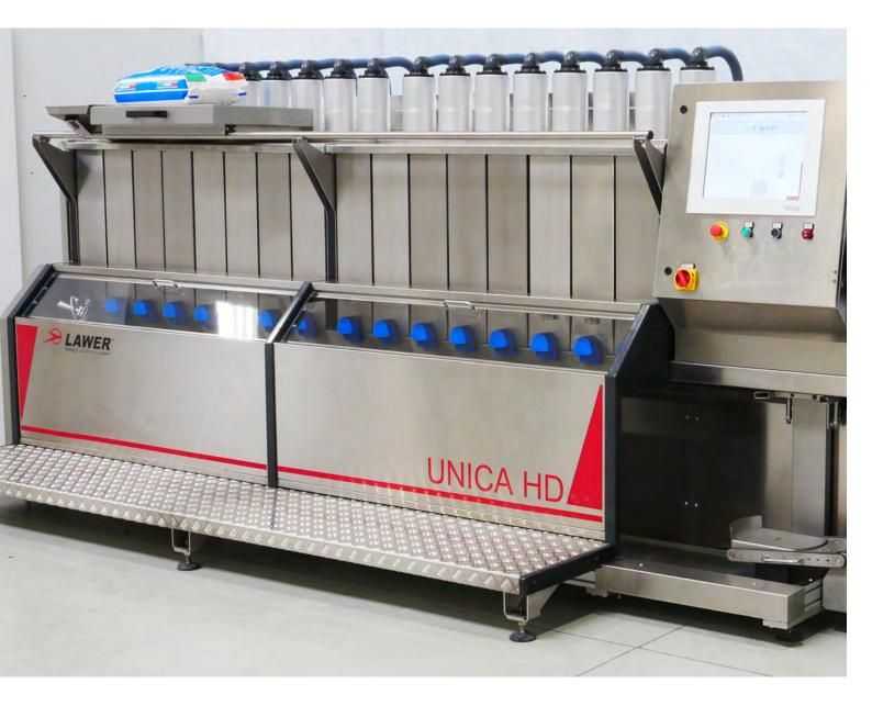
For **small-medium productions**, the solution is **UNICA**; this system has been designed and patented to organize production in an innovative way, by automatically weighing the powder ingredient components of recipes and batches in different processes of the food preparation industry.
