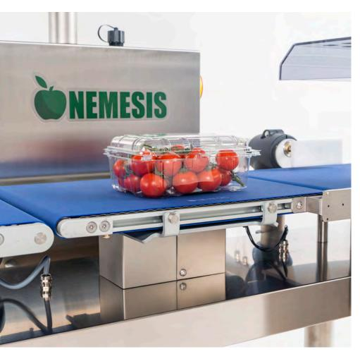
with MID-certified results, products from 5g up, with 0.2g accuracy and conveyor belt speed up to 100 m/min.
