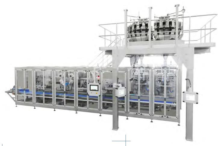
TWIN vertical packaging machine integrated with corrousel Model MCRV-D, reaching 120 bpm, combined with 28-heads multi-head weigher.
