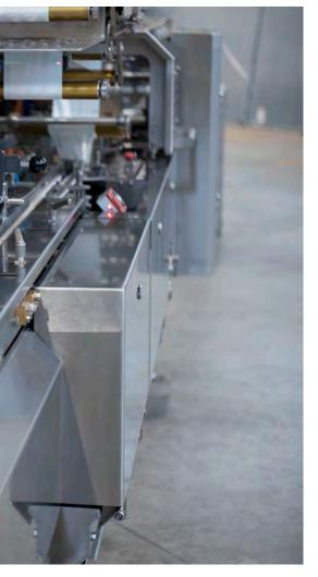
ZERO5BMF: a high performance flowpacker, with 'BoxMotion' transversal sealing technology. It is one of the fastest machines on the market, reaching speeds of over 300 pieces / min.
