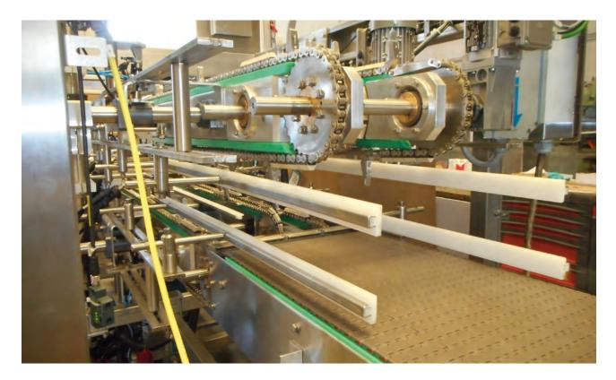
materials, it has small dimensions and is equipped with a curvilinear multi-way entry with divider block. This configuration makes the operator's work easier, ensuring ease of access to the machine both during its functioning and during ordinary and extraordinary maintenance.
