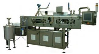
family, respecting the memory and the groove traced by a great inventor and creative genius. Aseptic fillers ALCOS can be two heads or single head. They can operate with any type of aseptic bag in the widest range of filling, with 2-3-5-10-25-220 L bags and even 1000 L, all can be packed in a single machine with interchangeable filling capacity.
