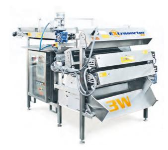
tem and to the ejecting unit. The exclusive electro-pneumatic ejection system with "fingers" has proven to be the most effective for average dimensioned product, such as industrial tomatoes. For products of smaller dimension, such as small tomatoes ("cherry") and red pepper,
