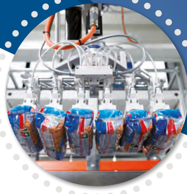
TWIN ROBOT robot for high-speed wrapping of flow pack packages in shrinkable film
