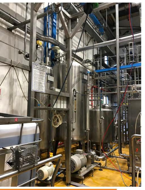
Gear metering pumps in a food beverage Plant
