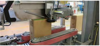
Carton Packer) suitable for American cardboard case (RSC) with a "pick & place" system for inserting the bulk product into the package.
