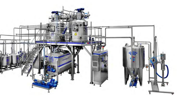
Tomato mix, ketchup, jam processing line with ingredient feeding and mixing system pre-built and FAT tested before shipping
