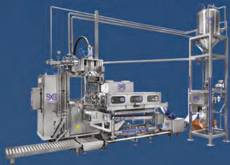
SINGLE HEAD ASEPTIC FILLER FOR WEB FILLING OF 3-20 LITERS BAGS SEMI - AUTOMATIC 220 BAGS IN DRUM FILLING
