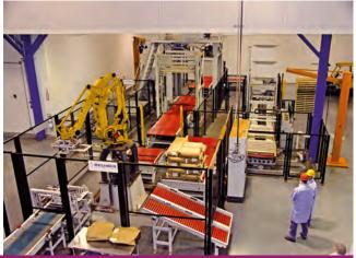
The packaging system at a glance: as general contractor, BEUMER Corporation has installed a complete packaging system, conveying systems and a bagging system.
