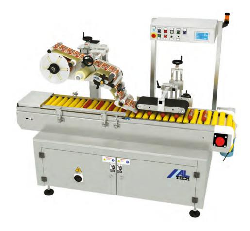
he wraparound labelling is a very common application in the packaging world, and for this ALTECH has developed a line of automatic systems able to adapt and apply wraparound labels on any cylindrical product. This labelling system, called ALline C, is extremely flexible and, thanks to its modularity, it can be customized in such a way that it assumes multiple configurations capable of satisfying the most diverse labelling requirements.
