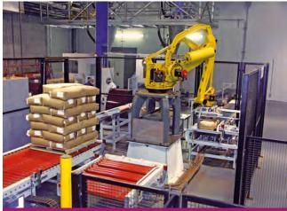
The BEUMER robotpac in use: the palletised stacks are characterised by an excellent stack quality.
