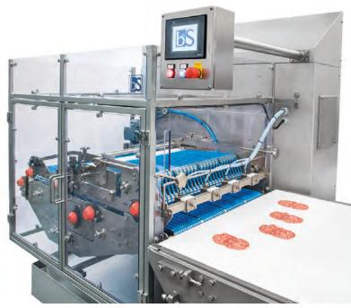
B.S. reel is not a standard machine: it can be manufactured in single or multiple line, adjusting the operational width according to the customer's needs. This machine can also be equipped with a single motor or an independent motorization for each raw. Moreover, it can be installed into any production line.
