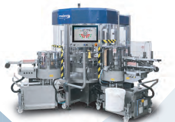
Example of configuration with cold glue stations
