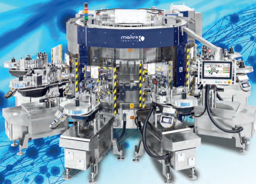
MAK machine configuration with HS2 adhesive units
