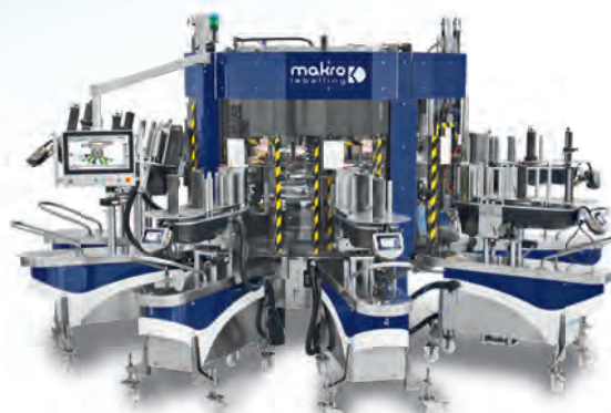
MAK machine configuration with HS SLIM adhesive units
