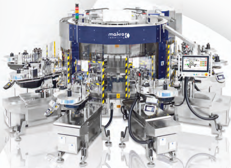
MAK machine configuration with HS2 adhesive units
