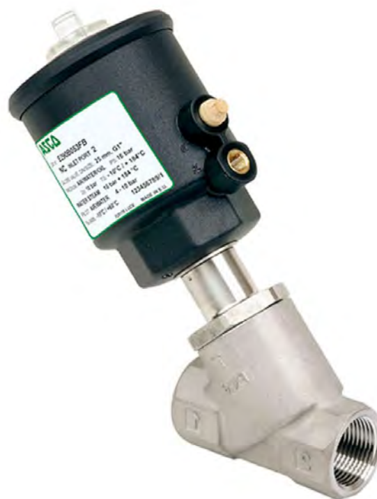
The ASCO Series 290 is a pressure-operated, direct-acting, angle seat-body valve built for demanding applications such as fermentation
