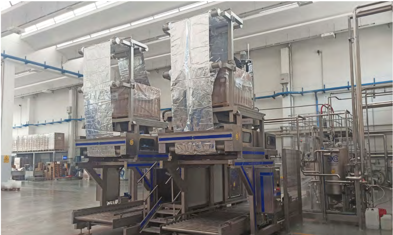
Double head aseptic filler for palletized bags 220 liter in drums, small bags 3 – 5 – 10 - 20 liters with automatic bags loading system and automatic filling of product - no operator needed. – Patented System – great filling speed.
