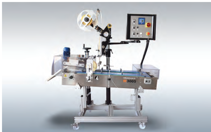
M3005 S FOR LABEL APPLICATION ON SALAMI
