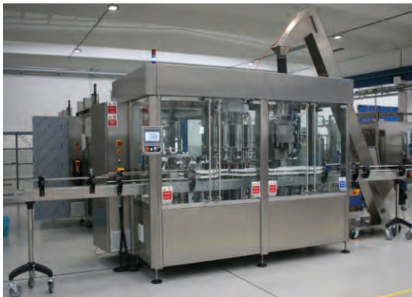
Rotary Filler with 12 valves, counter-pressure electro pneumatic technology. With Double Pre-Evacuation system suitable for Beer
