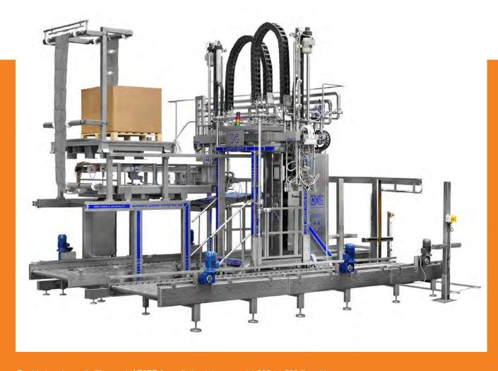
Double head aseptic filler mod. AF2PD for palletized drums and 1.000 / 1.500 liters bins with automatic loader for 5-10-20-220 liters bags.
