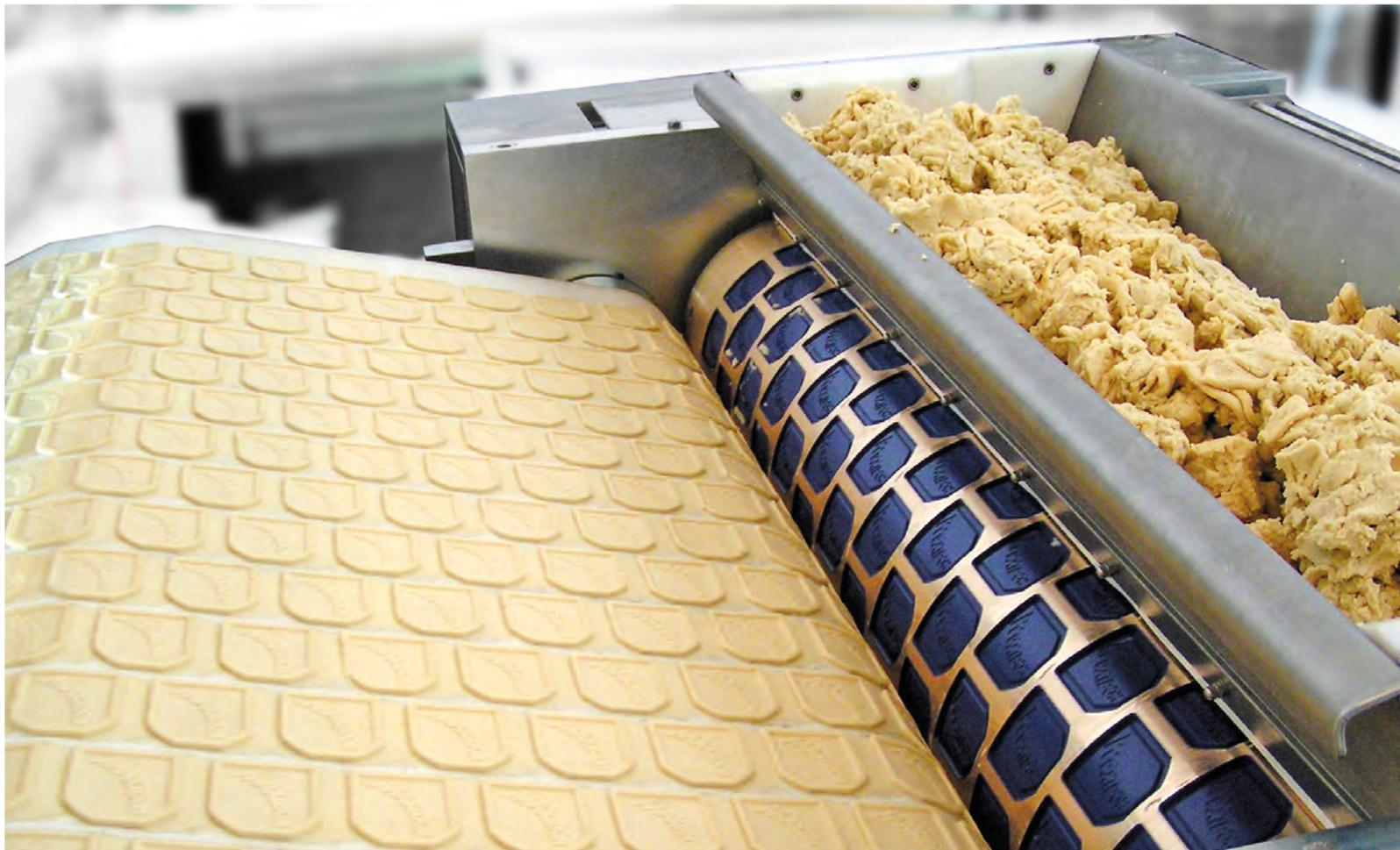
dough making and moulding, to baking, to the final product wrapping.
