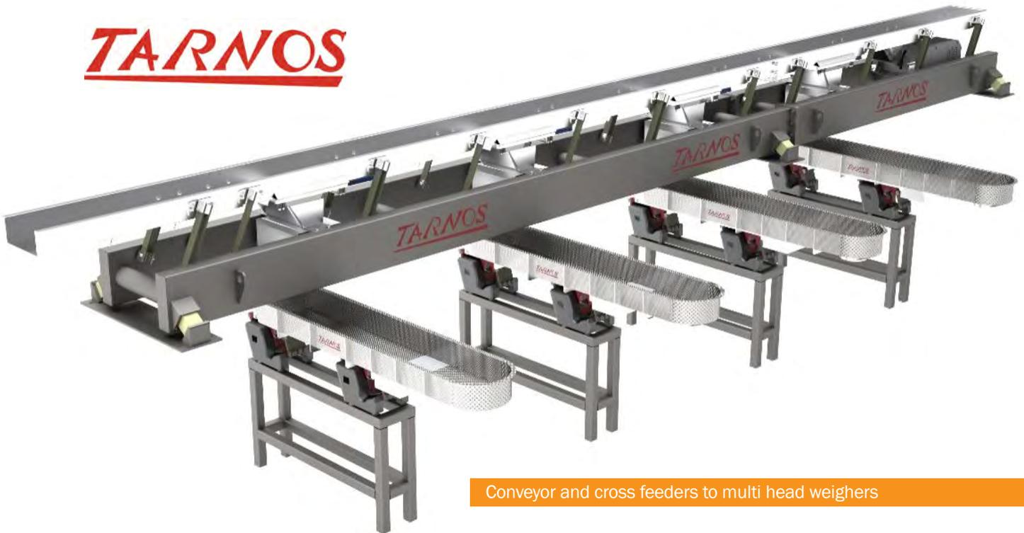
Conveyor and cross feeders to multi head weighers
