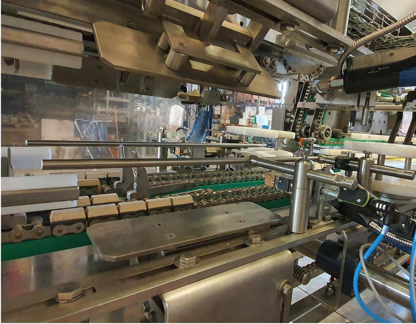
other stainless materials, it has small dimensions and is equipped with a curvilinear multi-way entry with divider block. This configuration makes the operator's work easier, ensuring ease of access to the machine both during its functioning and during ordinary and extraordinary maintenance. The WA30 Continuous Wrap Around case packer is
