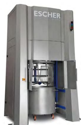
Line with independent tool movement, with individual speed regulation and the possibility to reverse the motion.
