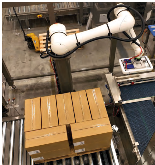
Solution for the pharmaceutical industry: a Cobot assembles a pallet of American cases labelled with a warehouse wrap-around label.
