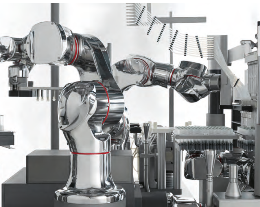
INJECTA 36 filling and stoppering
