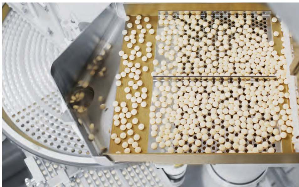
The patented Sombrero universal feeder, 3-row version
