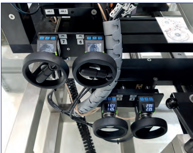
Figure 5: Size changeover using SIKO position indicators on a Track & Trace system in pharmaceutical manufacturing
