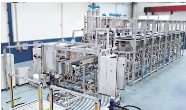
der products with the manual weighing assisted by a PC. In this way, according to the recipe, the system drops the right box and transfer it to the weighing position, where the operator, guided by the PC can dose the product.
