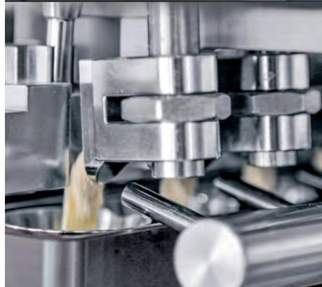
Volumetric dosing system for granules
